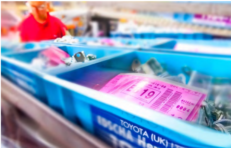
A kanban card on parts in a Toyota factory in the UK
